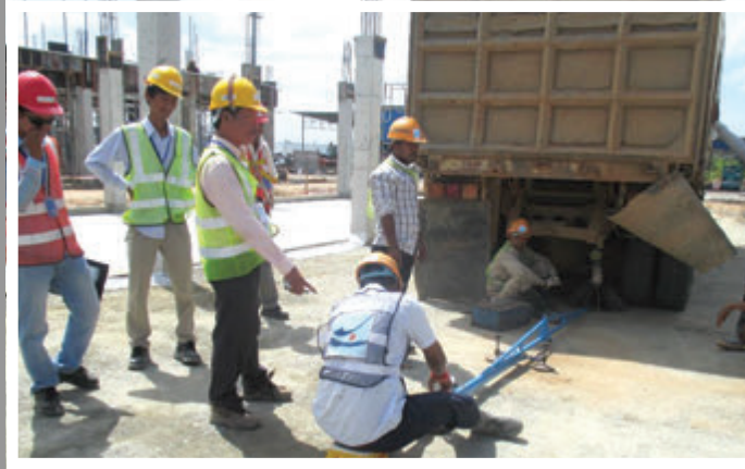
Compaction Field Test: Sand Cone Test with Vinci QC Team
